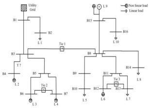
Fig.2. Single line diagram of the IEEE 16-bus test system
