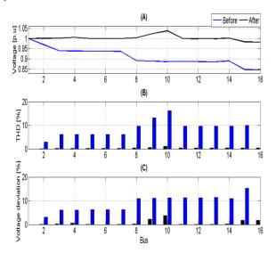
Fig.3. System performance before and after the D-STATCOM installation in the 16-bus test system; (A) Bus voltage, (B) Bus THD (C) Voltage deviation.
